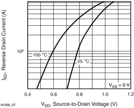
Fig. 7 - Typical Source-Drain Diode Forward Voltage
